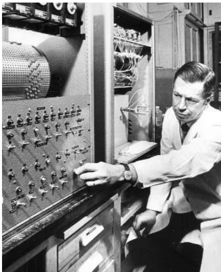
A practical solution for peptide synthesis. In this 1969 photo, Merrifield adjusts an early version of his peptide synthesizer.
